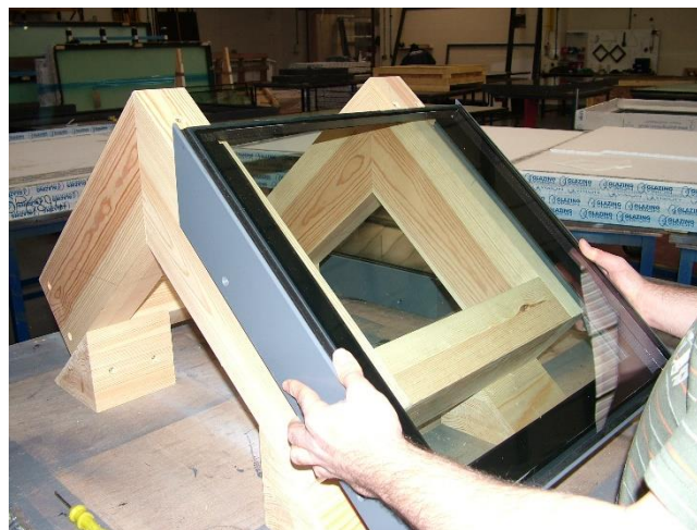
Figure 8 – Installing the first half of the unit
