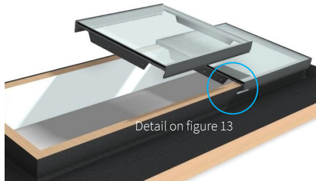
Figure 12 – Joining plate inserted
